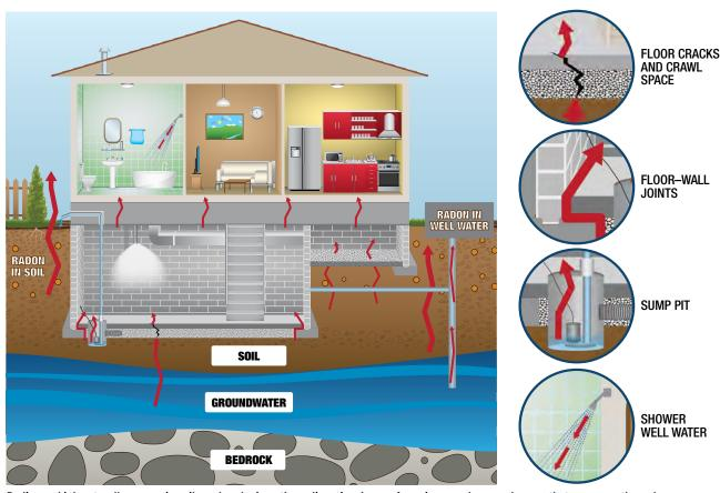
Radium, which naturally occurs in soils and rocks from the radioactive decay of uranium, produces radon gas that can move through the soil into a home or other building through these common entry points. Because the air pressure inside a home is often lower than the pressure in the soil around the foundation and basement floor slab, radon is easily drawn into a home due to these air pressure differences.
